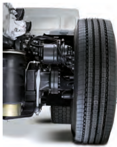
AIR SUSPENDED REAR CHASSIS offering increased stability and better protection of goods.
