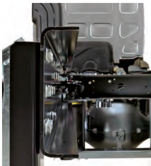
CHASSIS SIDE MEMBERS in high tensile steel.
