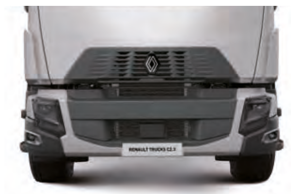
PLASTIC BUMPER (C 2.3) WITH STEEL CORNER PIECES for greater resilience.
